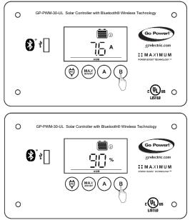
Push the **B Button** to show the PV charging current for battery 2. The GP-PWM-30-UL will begin to limit the current as the battery 2 reaches a full charge.
