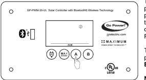
To select the charging profile of battery bank 2, press the **B Button** to toggle through the profile options: Sealed/Gel, AGM, Flooded, or LFP.
