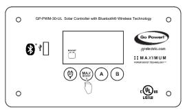
To activate, hold the **MAX BOOST Button** for 3 seconds. As long as there is full sunlight present, your battery voltage will be boosted (to 14.4 VDC for Flooded, AGM and LFP; and 14.1 VDC for SEALED/GEL) for 30 minutes regardless of the battery's state of charge.
