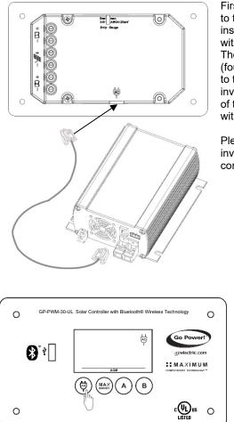
First, connect the inverter directly to the battery (follow the installation instructions included with the inverter). Then, connect the modular cable (found in the inverter remote box) to the remote terminal of the inverter <u>and</u> to the remote terminal of the GP-PWM-30-UL (marked with an **AC Plug symbol**).
