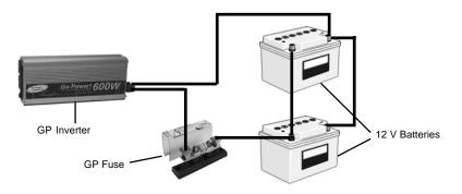
\*Installation using two 12 volt batteries.
