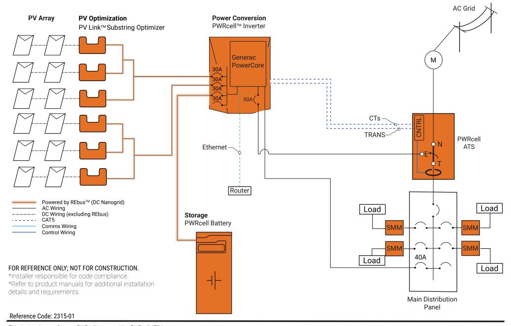
This design shows a Generac PWRcell system with a PWRcell ATS in a whole home backup configuration. Use this system configuration to provide backup power to the main service panel loads using Generac Smart Management Modules (SMMs) for load shedding in accordance - 6 PV Links with NEC 702.4(B) and Article 220.
