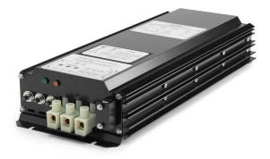
Model 6929 is designed to meet the emerging need to charge lithium battery banks from 12V systems. Model 6929 will output 45A @ 29V in full charge mode and can be operated while load is drawn from the battery bank being charged. Off the shelf units are ideal for use with lithium iron phosphate batteries. Model 6929 is microprocessor controlled and can be programmed at factory for operation with other battery types.
