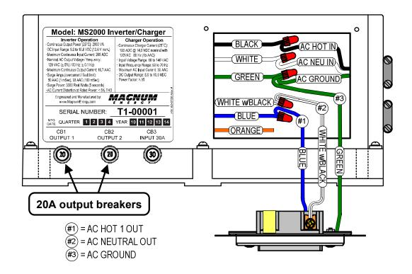
Figure 2, AC Output Wiring for MS2000-20B
