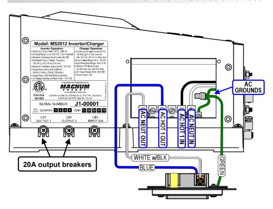
Figure 1, AC Output Wiring for MS2012-20B
