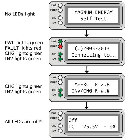
\* If the Power-up Always feature is enabled and DC is reconnected to the inverter, the inverter will turn on automatically once the self test is complete.
