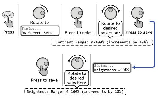
Figure 3-15, SETUP: 08 Screen Setup Selections
