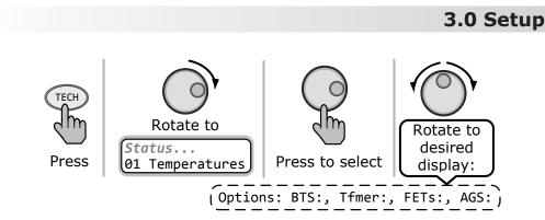
Figure 3-16, TECH: 01 Temperatures Display
