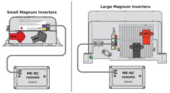
Figure 2-2, Remote Control Connections
