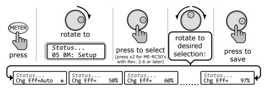
Figure 8-2, Adjusting the Charge Efficiency Setting
