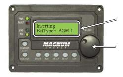
Rotate the **SELECT** knob to the desired setting. When the bottom line shows the desired setting:
