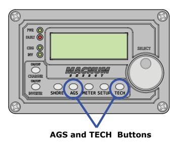
Figure 7-1, ME-RC's AGS Configuration Access Buttons
