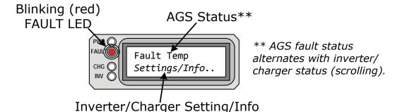
Figure 7-4, Example: AGS Fault Message on ME-RC Remote
