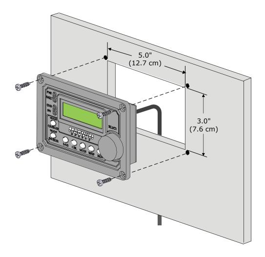
Figure 2-4, Flush Mounting the ME-RC
