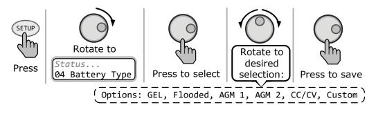
Figure 3-9, SETUP: 04 Battery Type Selections
