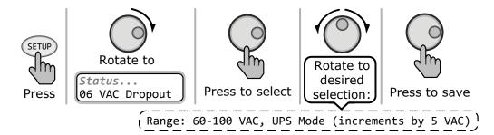
Figure 3-13, SETUP: 06 VAC Dropout Selections
