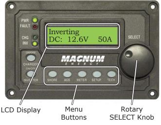
Figure 3-1, Front Panel Setup Features
