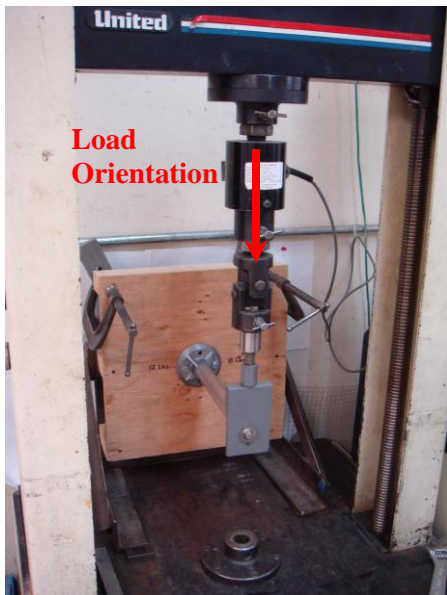
Figure 2a. Shear Perpendicular to Rafter
