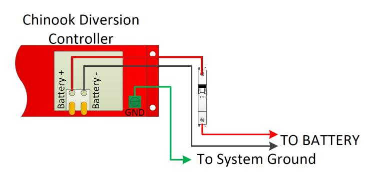
The terminal block for the positive and negative battery wires can accept #10-24 AWG. It is recommended to use #10 wire for this connection.
