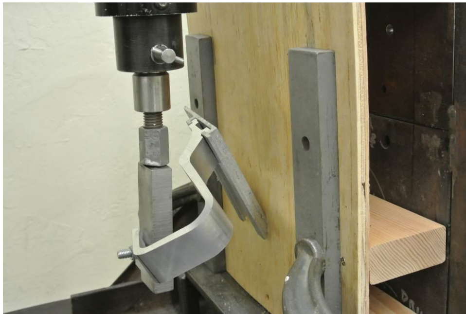
Figure 4b. Typical Failure Mode
