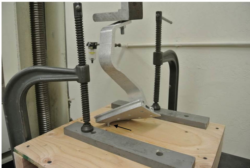
Figure 2b. Typical Failure Mode
